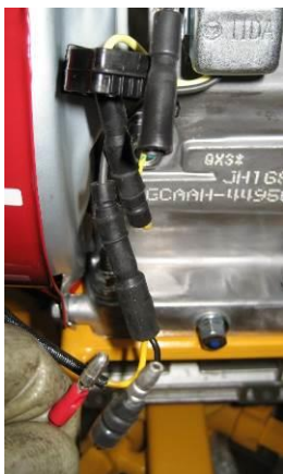
1 DISCONNECT THE BLACK WIRE FROM THE SPARK
